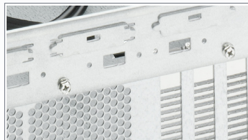
Break-outs for rear-side interfaces
